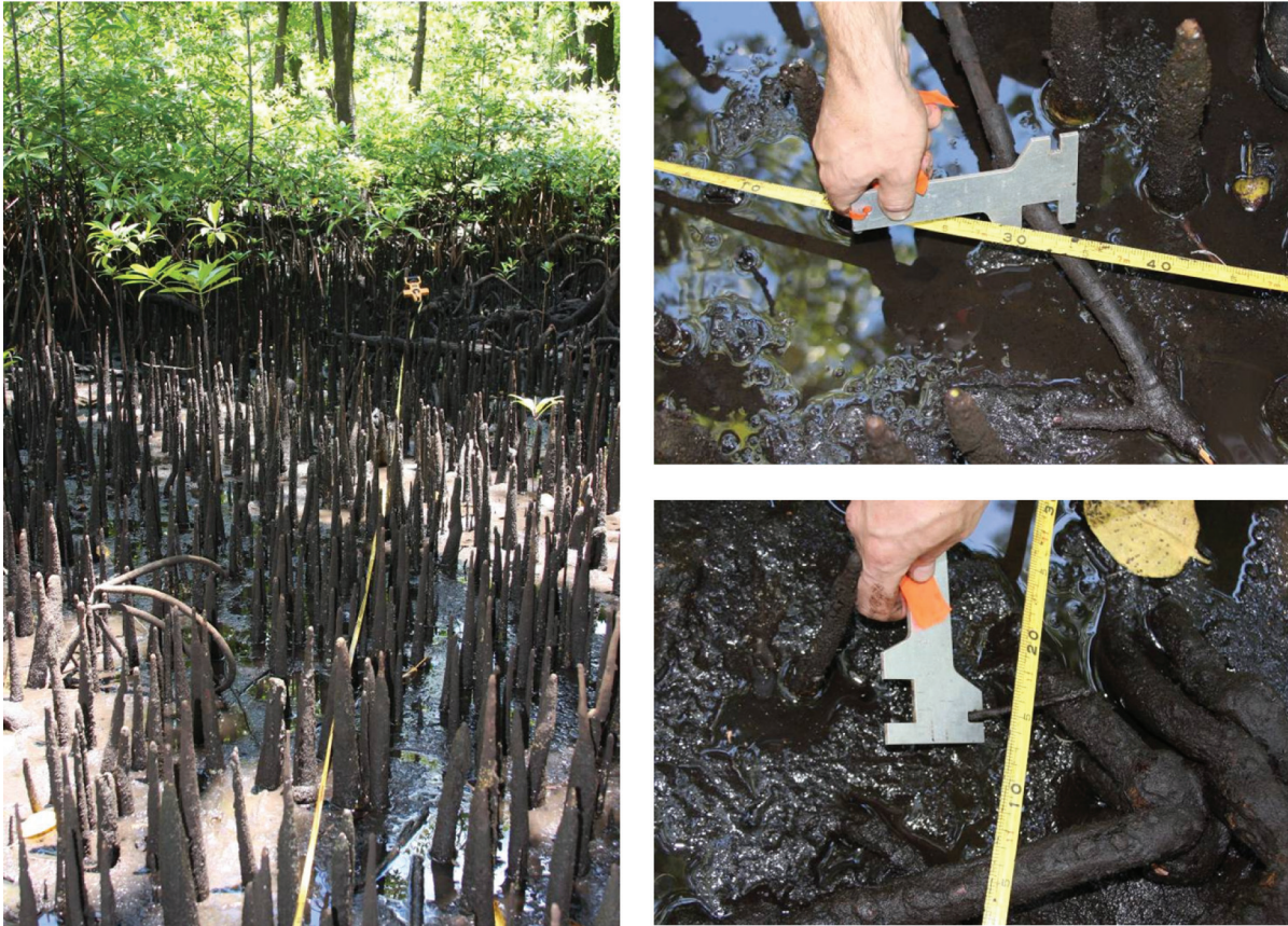
Figure 14. Example of a woody debris transect tape in a mangrove (left), and using the down-wood gauge to classify pieces by size (right). The upper right piece is a medium class; the lower right piece is small class.
